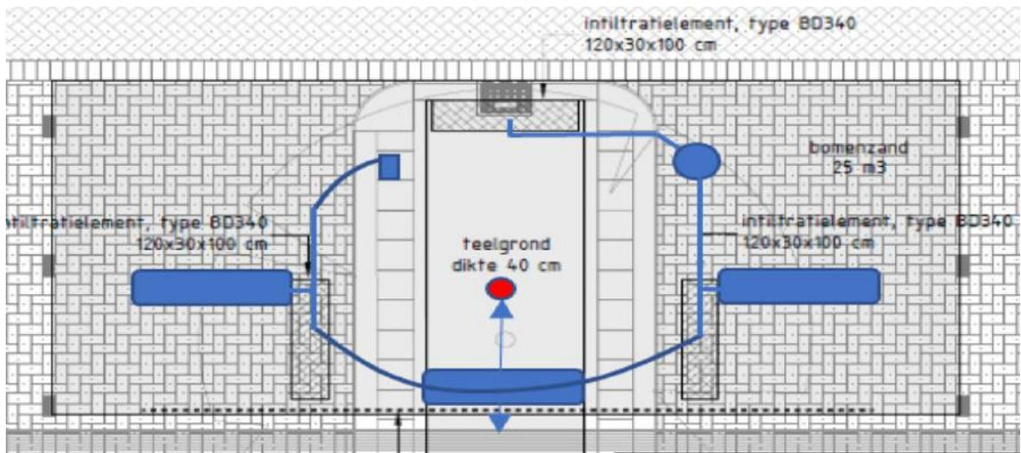
For some tree pits, a four-module array was used increasing the capacity by a third
