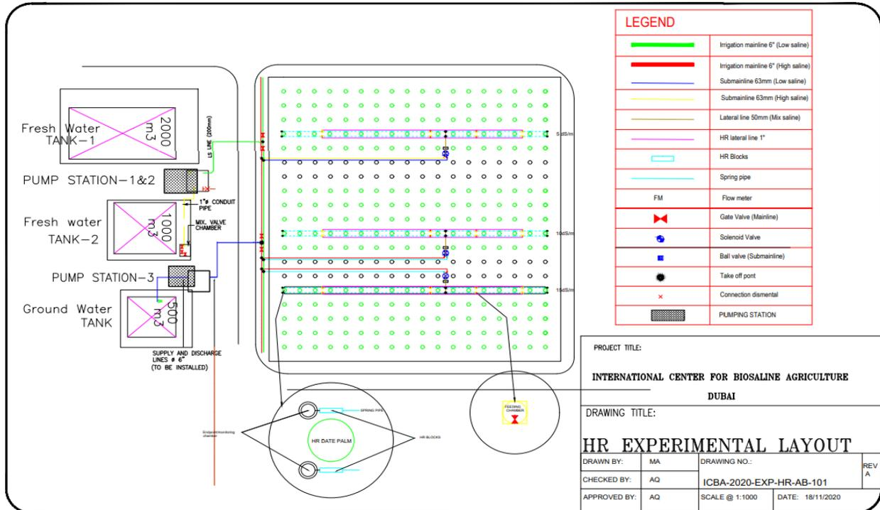
Figure 1: Hydrorock subsurface irrigation system installed at ICBA station.
