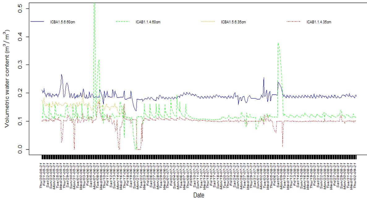
Figure 8. Volumetric water content ( $m^3/m^3$ ) at the end of the line at 60 cm and 35 cm soil depths.
