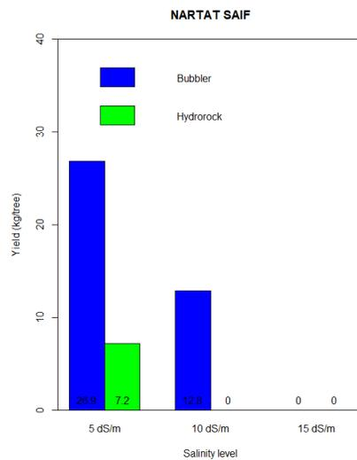
Figure 15. Fruit yield (kg/tree) by the bubbler and Hydrorock systems in three salinity levels for NARTAT SAIF variety.
