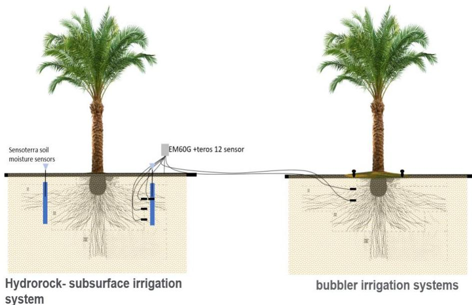
Figure 2. Schematic view of HydroRock and Bubbler irrigation systems installed at ICBA station.
