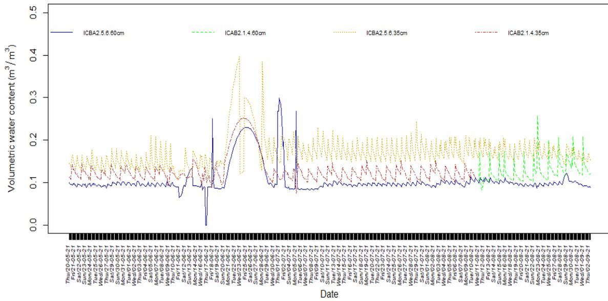
Figure 7. Volumetric water content ( $m^3/m^3$ ) at the beginning of the line at 60cm and 35cm soil depths.
