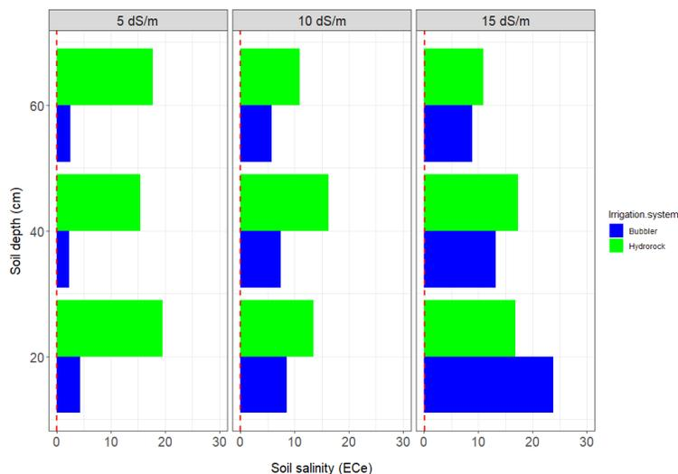
Fig. 26. Soil salinity for bubbler and Hydrorock systems at three soil depths (Sept. 20, 2021).
