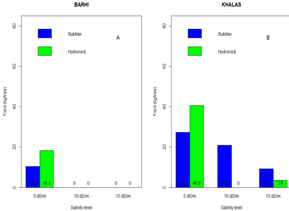
Figure 10. Fruit yield (kg/tree) by the bubbler and Hydrorock systems in three salinity levels for (A) BARHI variety and (B) KHALAS variety.
