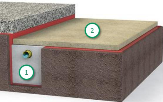
① Hydrorock BD element (L 1200 x H 360 x W 330 mm) as perimeter drainage system
