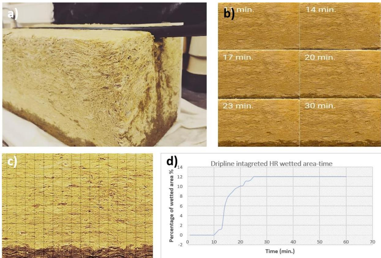
**Figure 12** Distribution of water within a stand-alone Hydrorock pressure compensated block over time during an irrigation event.
