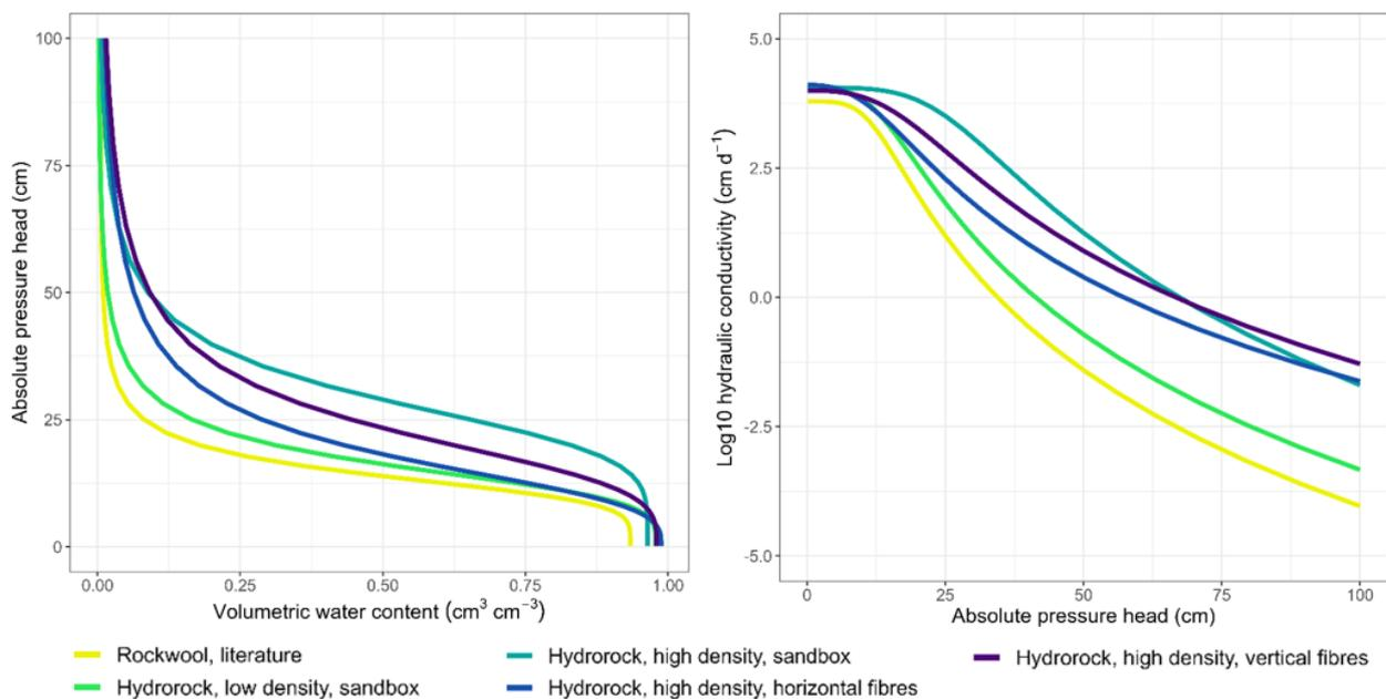
**Figure 5** Water retention characteristics (left) and Hydraulic conductivity characteristics for different configurations of HR blocks.
