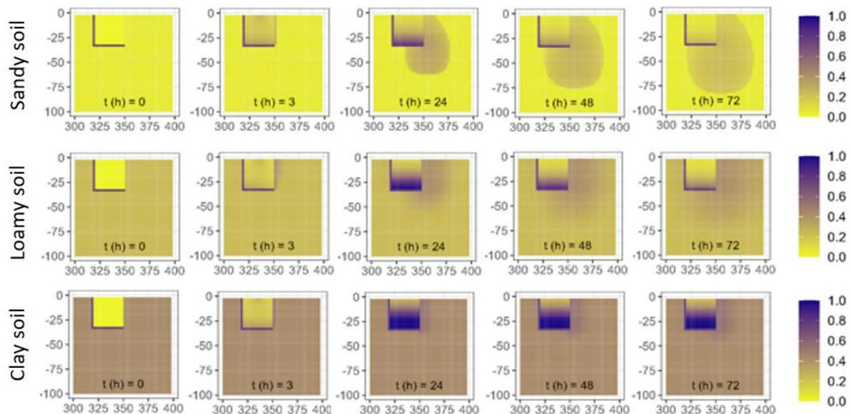
**Figure 15** Simulation of a single irrigation event using a D112 IR low flow (2.3 l/h) control block under three different types of soils: sandy, loam and clay.
