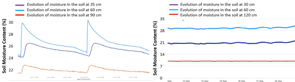
**Figure 16** Soil moisture behaviour over 144 hours in the Hydrorock system (soil), at 3 different depths for a sandy soil with non-control flow block (left) and a loamy soil with high flow control block (right)<sup>4</sup>.
