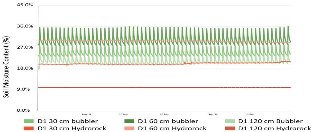
**Figure 31** Evolution of soil moisture levels for date palms irrigated with Hydrorock blocks (red) and bubbler (green) at different depths (30, 60 and 120 cm).
