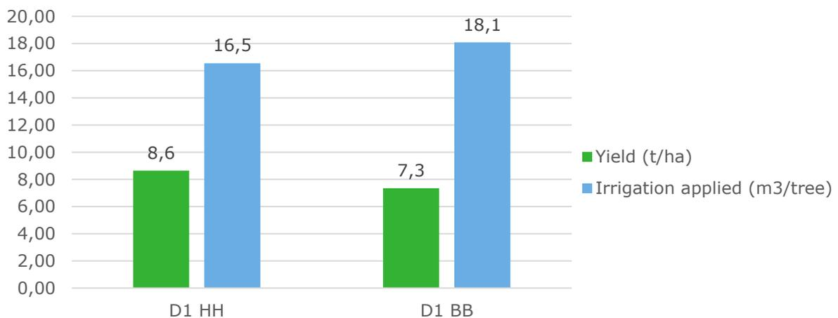
**Figure 30** Total water applied (m3/tree in the summer season) and yield (ton/ha) for date palms irrigated with Hydrorock blocks (HH) and bubbler (BB).
