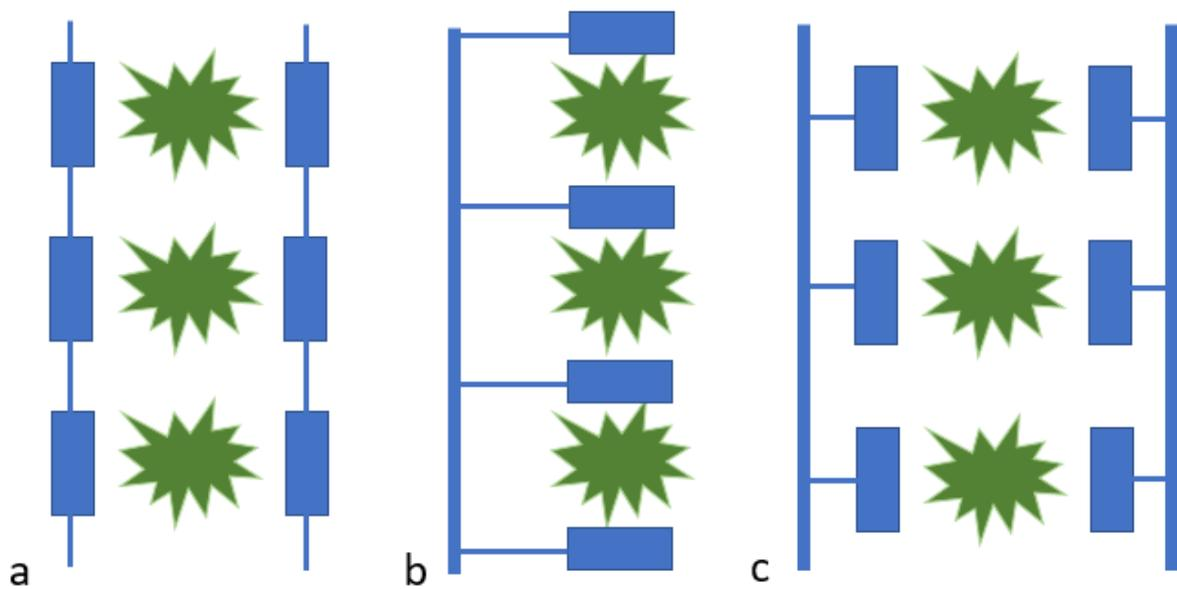
**Figure 8** Different configuration option: a) in line with two elements per tree and blocks connected to a lateral pipe; b) in parallel, with two elements per tree and directly connected to a main/secondary pipe; c) in parallel, with two elements per tree and connected to a lateral pipe.
