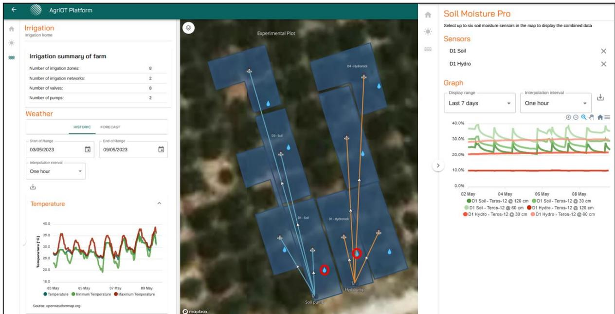
**Figure 18** Agriot platform developed by SFS. Real-time data from soil moisture sensors as well as weather information can be visualise and downloaded for further analysis. Example showed for the pilot developed in Bahrein at the Hoarat A’ali farm.
