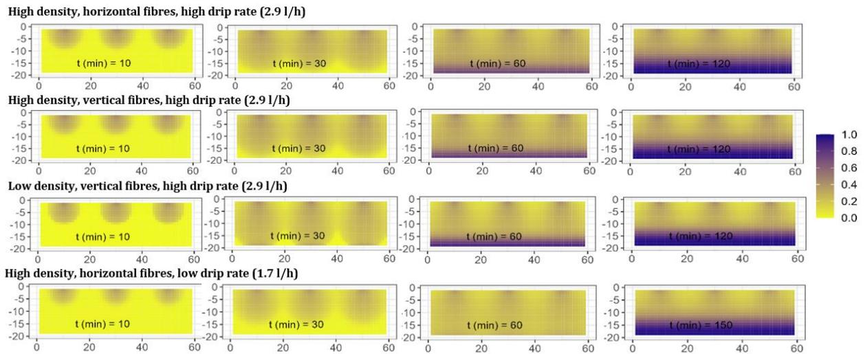
**Figure 11** Distribution of water within the Hydrorock block on a single irrigation event using a D112 IR flow control block with different rockwool properties (density and fibre direction).
