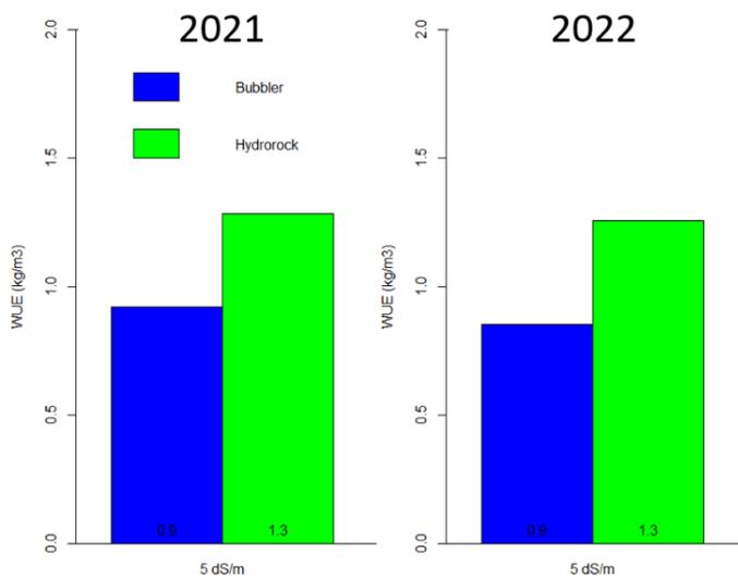
**Figure 23** Water use efficiency of date palms irrigated with Hydrorock (green) and with bubblers (blue), for 5 dS/cm.
