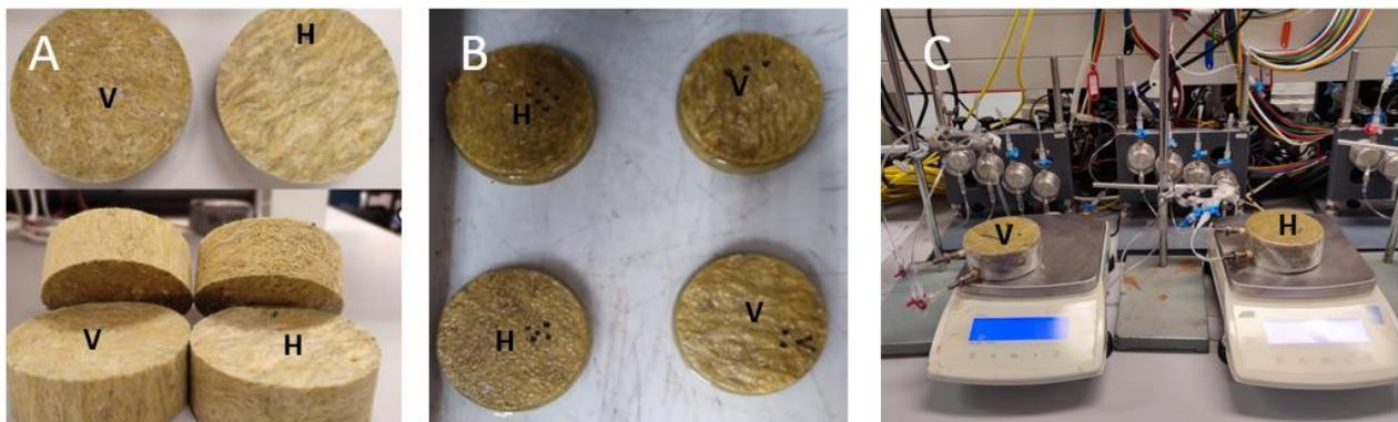
**Figure 3** Hydrorock samples used for Wind's evaporation method. A) dry samples; B) saturated samples; C) experimental configuration (Arikan. 2023).
