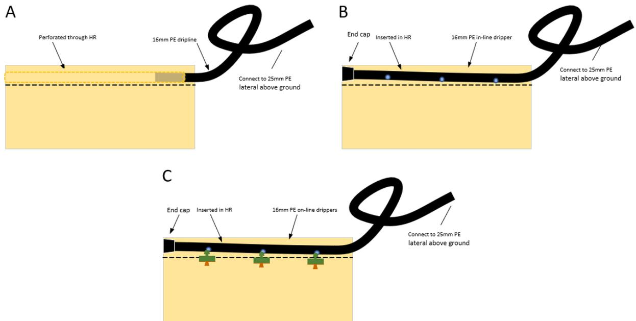
**Figure 7** Potential configuration of Hydrorock blocks, depending on their capacity to control the flow of water.
