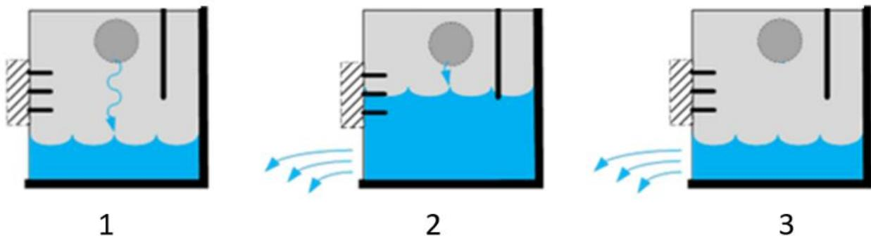
**Figure 10** Schematisation of the functioning of a Hydrorock block.
