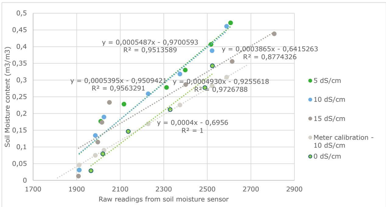
**Figure 26** Linear calibration curves of soil moisture sensor signal for 4 water qualities (0, 5, 10 and 15 dS/m) and comparison with the generic calibration curve proposed by the provider.
