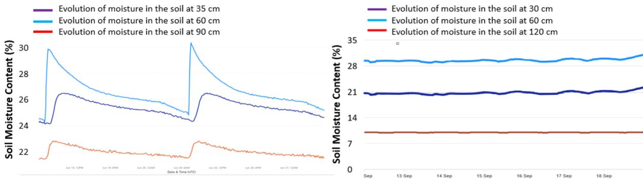
**Figure 16** Soil moisture behaviour over 144 hours in the Hydrorock system (soil), at 3 different depths for a sandy soil with non-control flow block (left) and a loamy soil with high flow control block (right)<sup>4</sup>.
