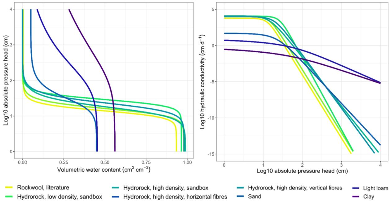
**Figure 6** Water retention characteristics (left) and Hydraulic conductivity characteristics for different configurations of HR blocks and different type of soils.
