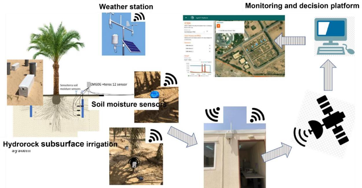
**Figure 17** Potential layout of an operational irrigation system with HR blocks in a date palm plantation.
