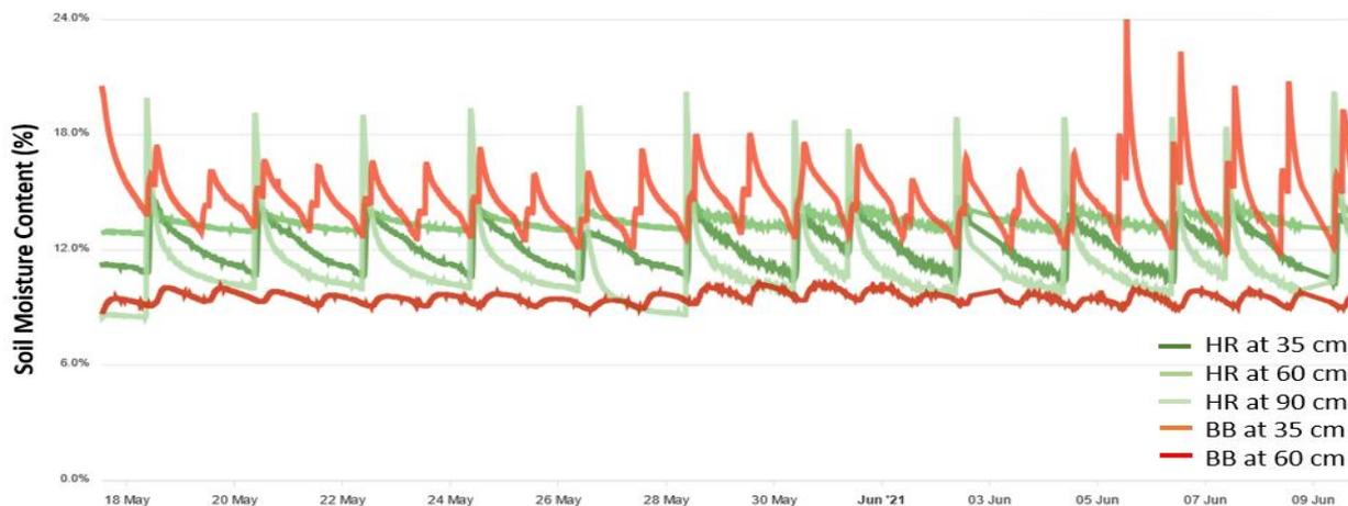
**Figure 21** Evolution of soil moisture at different soil depths for a date palm line irrigated with Hydrorock block (green lines) and a date palm line irrigated with bubblers (red lines). Data showed from 18 May 2022 to 10 June 2022.
