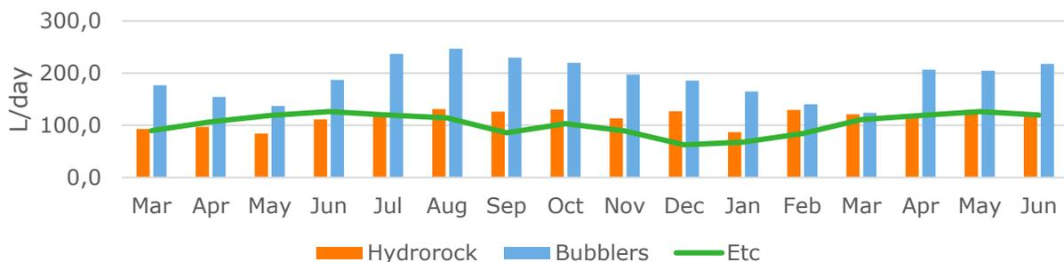
**Figure 20** ETC versus irrigation applied by Hydrorock and Bubblers in 5 dS/m (L/tree/day). Data from March 2021 to June 2022.
