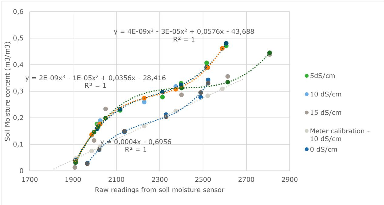
**Figure 25** Polynomial calibration curves of soil moisture sensor signal for 4 water qualities (0, 5, 10 and 15 dS/m) and comparison with the generic calibration curve proposed by the provider.
