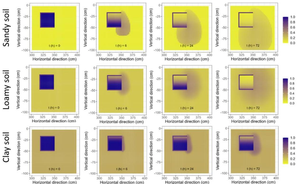
**Figure 13** Simulation of a single irrigation event using a D112 IR non-flow control block under three different types of soils: sandy, loamy and clay.
