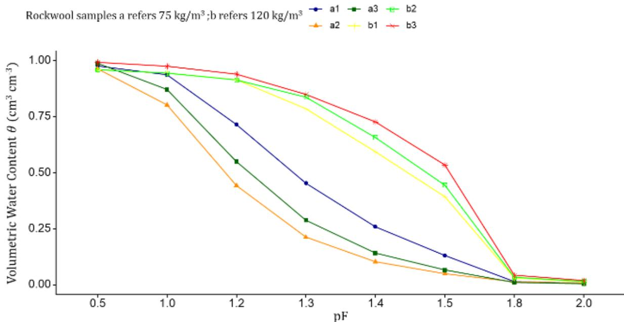
**Figure 4** High and low-density types of stone wool cylinder samples representing each sample's water content changes with suction between 0 to 2 pF.
