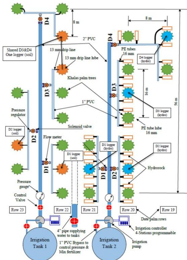
**Figure 29** Lay-out experiment date palms with sensor location.
