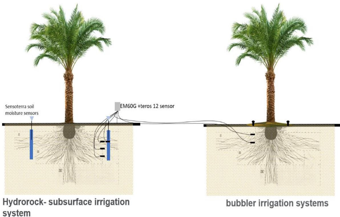
**Figure 19** Layout of HR blocks and bubblers and soil moisture sensors.
