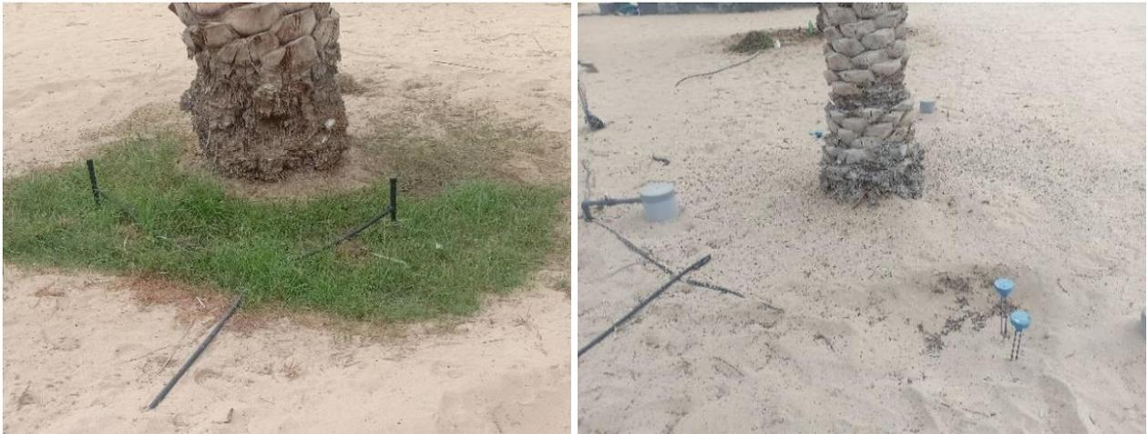
**Figure 27** Growth of weed under bubbler (left) and Hydrorock system (right).
