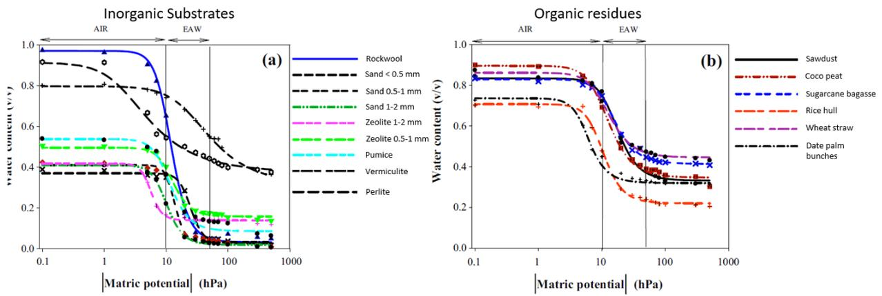
**Figure 1** Comparison of water retention curves of stone wool (rockwool) material with other potential inorganic (left) and organic (right) substrates (Banitalebi et al. (2019)). Values predicted by van Genuchten model.
