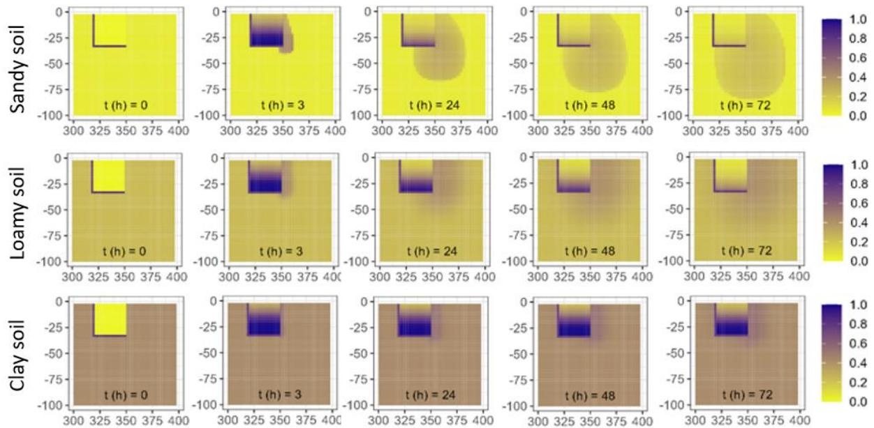
**Figure 14** Simulation of a single irrigation event using a D112 IR high flow (12 l/h) control block under three different types of soils: sandy, loam and clay.
